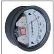
Differential Pressure Gauge Dryer make Magnethelic gauges are used to measure the pressure drop HEPA filter 0-500 Pa.
